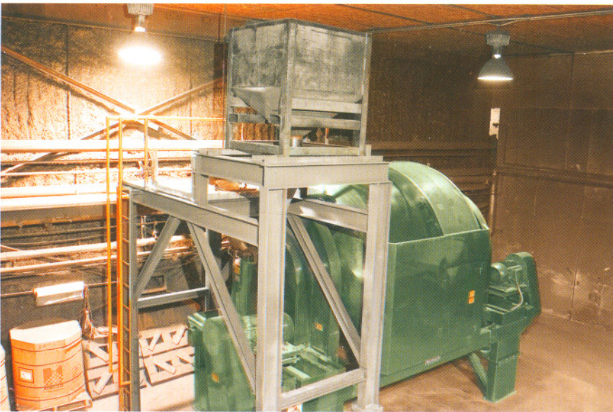
A structural stand holds a portable hopper and allows the company to add 5,000 pounds of material at a time into the blender's inlet, which is located about 9 feet above the ground.
