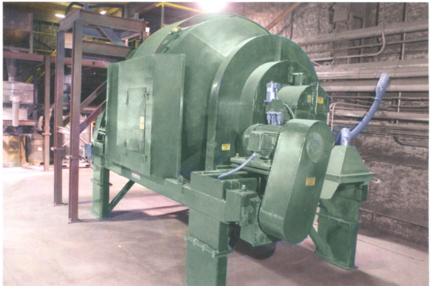
The 250-cubic-foot-working-capacity horizontal rotary batch blender can completely blend a 45,000-pound batch of metal powders in about 15 minutes.
